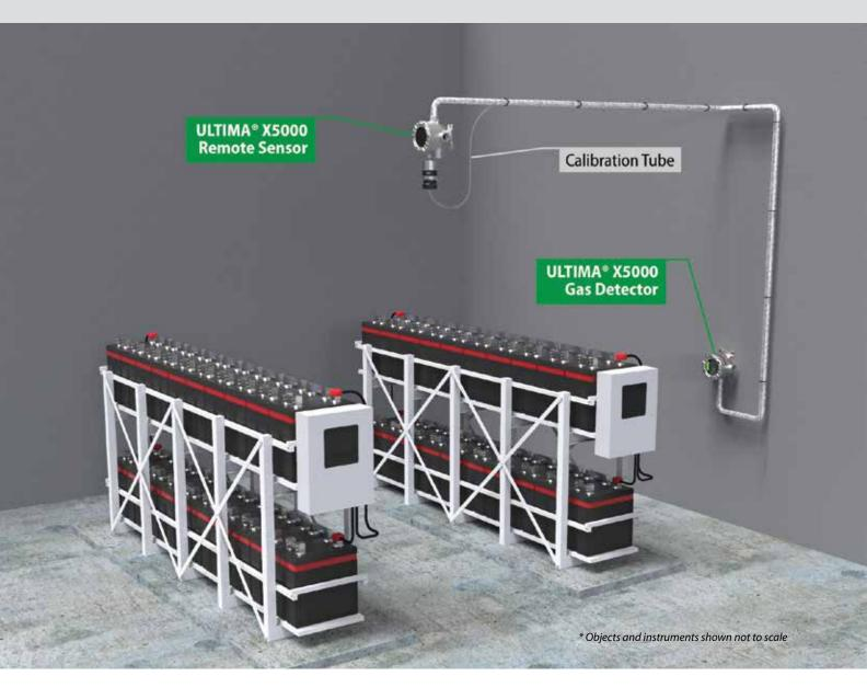
Battery back-up installations for equipment such as telecommunication stations and computers are normally situated in small rooms with little ventilation. This confined space provides an excellent opportunity for hydrogen to accumulate and reach combustible levels.
